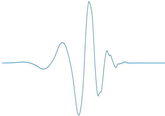
Figure 2. The profile of the Daubechies 5 wavelet. Based on our numerical analysis, a mother wavelet with vanishing moment 5 was found to provide a good representation for a RRAT’s pulse.
